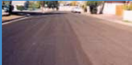
Phoenix, Arizona. Left side, TOR plus GTR after 2 years. Right side, SBS plus GTR shows asphalt stripping off the stone.
